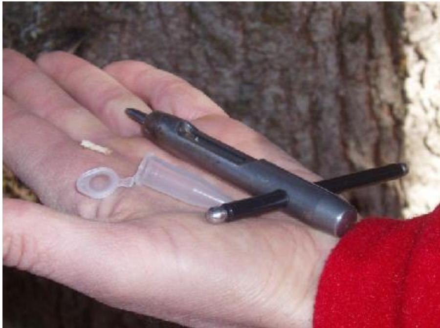
The microcore is ready to be kept in a storage container.
