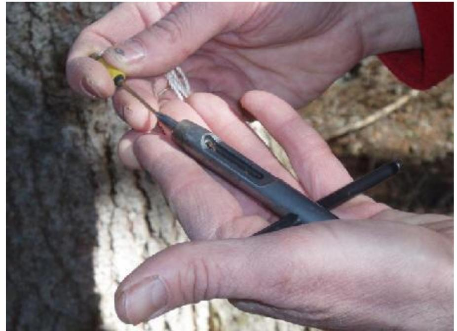
Use the “extracting needle” and push slightly the microcore on the top.
